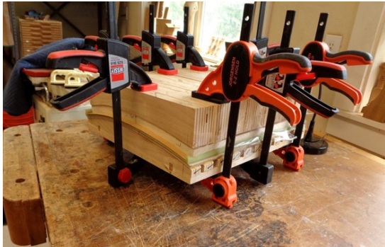
Form on which doors were laminated being used to veneer the fronts
