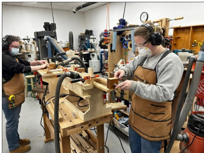
Miles and Allie turning tenons on the "router lathe" jig.
