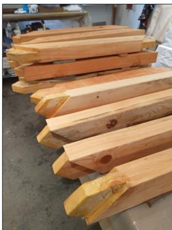
Knee braces after finishing
