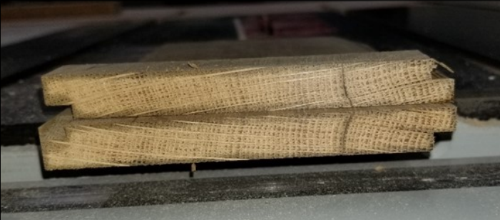
Fuming penetration after 24 hours.
