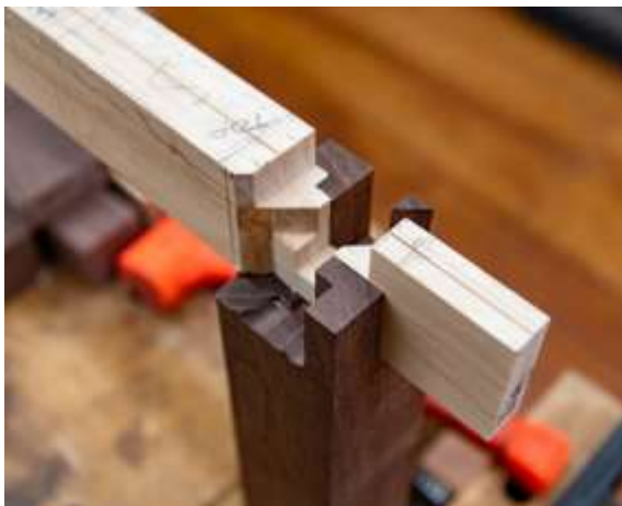
1 – Front chong bong to column
