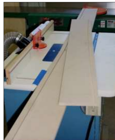
Figure 5. Trammel boards for gentle arc on router table
