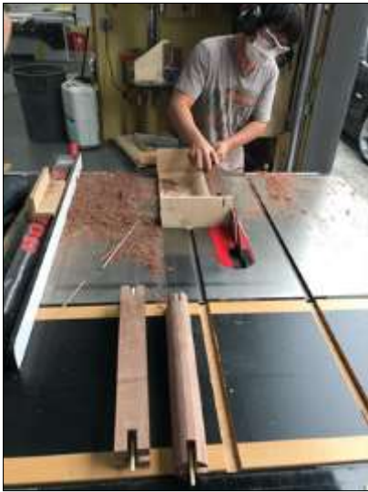
16 siding jig. Sector lines marked each 22.5 degrees on work piece and rotated to rip at each position.
