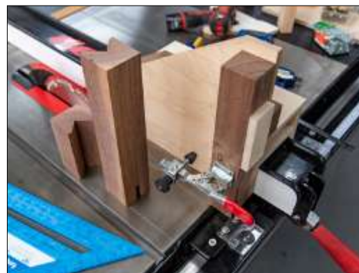
Tenon jig left side, with clamp blocks for diagonal slot cuts.
