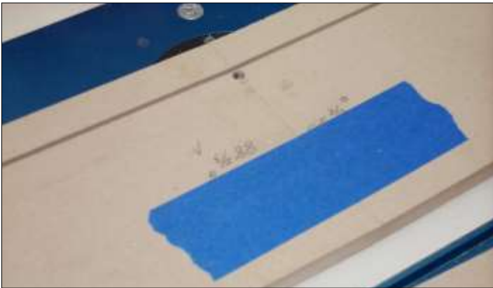
Figure 6. Spiral bit pokes up to route the arc. A guide bushing mounted in the route table plate (not visible) helps locate the grooved trammels
