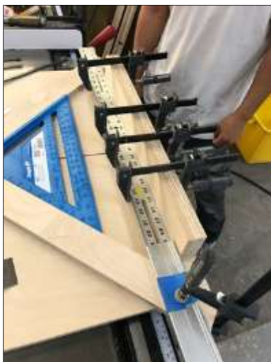
Sled fastened first to left base. Then clamped to straightedge and fastened to right base.
