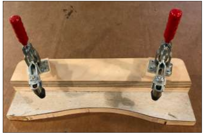
Photo 5: Clamping jig for holding rim segment part and pattern for routing the inside curve.
