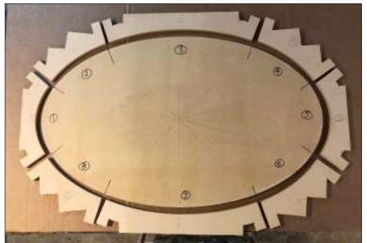
Photo 3: Pattern for the elliptical core with smaller patterns for each of the 8 segments that snug up to the core
