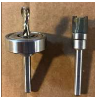
Photo 4: Special router bits used for creating a true complement pattern of the core ellipse.
