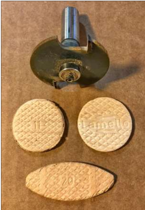
Photo 6: Author uses Lamello #11 biscuits (round) 36mm dia, compared to #20 biscuits (football) that are 23mm in width. Slots for the biscuits are cut with a 1 15/16" dia by 4mm slot cutting bit, shown.
