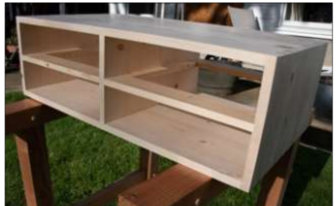
This photo and on page 11 show front and the open back of runner joint prior to installing case back.
