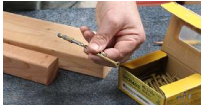
The feel test. If you roll a screw and a drill bit between your fingers, you can feel if they are roughly the same size, which is what you need for a clearance hole.
