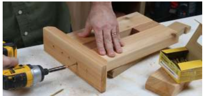
Simple, strong joinery. You don't always need complex joinery. To assemble the pedestals for a garden bench, I drilled clearance holes in the top pieces and pilot holes into the end grain below to make the screws super-secure. In fact the whole bench is joined with screws and glue, and you'd never know it.
