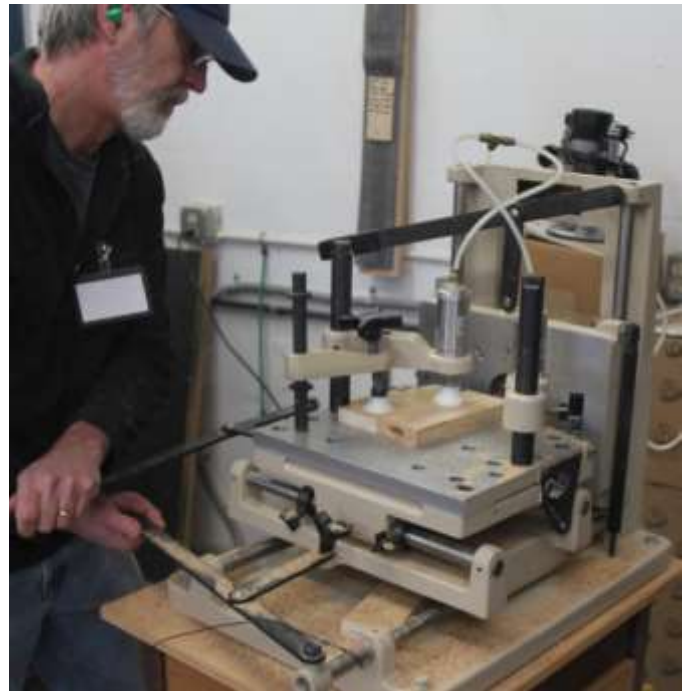
Commercial Multi-router made very fast work of mortis-
