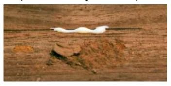
sanding sawdust from a nearby pile into the glue and massage it into the crack. Leave it to dry. I've tried pre-
