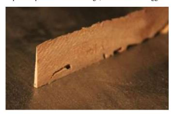
Capturing this piece as the saw cut finishes can be an exercise in itself. You need a tight fitting zero clearance throat plate so the sliver doesn't disappear into the innards of the saw's dust bin. It may want to fly off the table. This is one time it's ok to stand in front of it to capture it.
