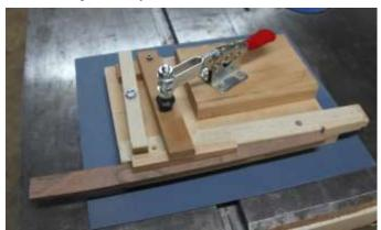
Safe to use, it's a rip on the table saw. Little finger hooked over the rip fence, firm grip on the clamp. If they were a little longer, the offcust could be chopsticks.
