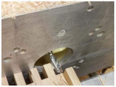
The box joint is ready to assemble.
