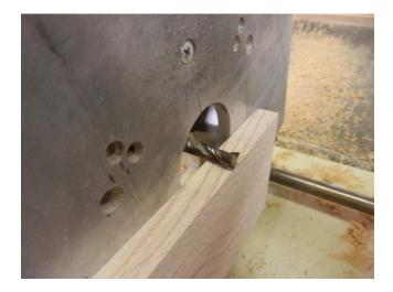
**Set up the template**. There is at least a couple of ways to accomplish the zeroing of the template.
