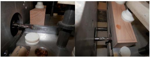
Use a test piece to check accuracy of all measurements. Be sure to lock all travels that need locked and stops set tight so they can't be moved.
