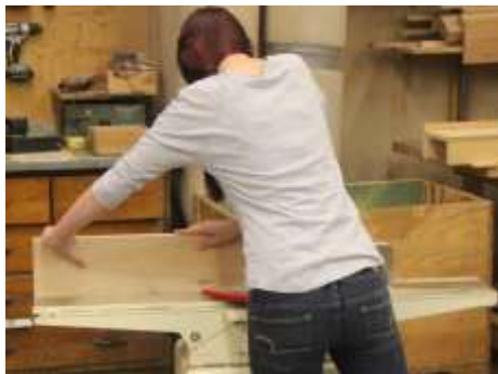
Jointing skirt boards
