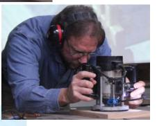
adds some sanding sawdust the color of the inlay, mixing it in the glue and spreading it to the sides. When the glue squeezes out, it fills any voids with sawdust. Awesome! Thanks, Marcus.
