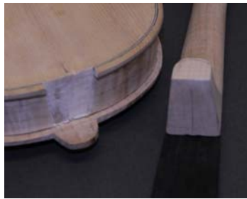
Cutting the mortise
