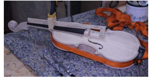
Gluing on the neck
