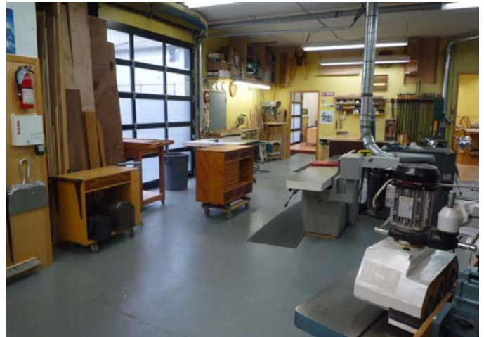
LR: Jointer, planer, shaper with power feed
