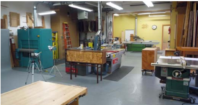
Two machine rooms. LR: wide belt sander, planer, shaper, (hidden) jointer, sliding table saw (far room), SawStop
