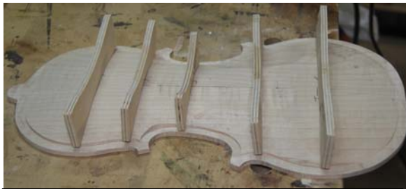
Using templates. Longitudinal and transverse
