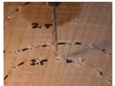
23 Drilling reference holes
