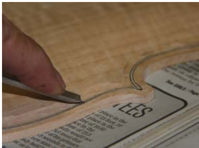
19 Cutting the channel
