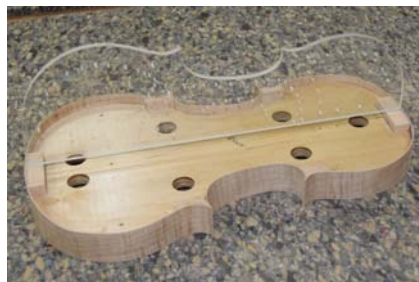
Pattern & mold. Ribs already on.
