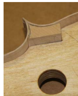
Corner block with ribs
