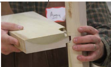
Testing the mortise for a press fit
