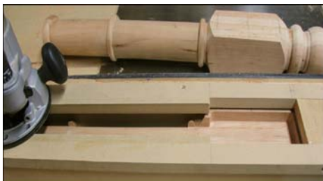
3. Routing using the template
