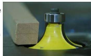
Fig 1. No bearing contact
