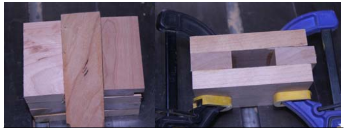
Handle for alignment, removed while the glue dries.
