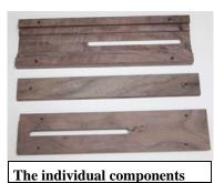
This design uses a double sliding joint with three components.
