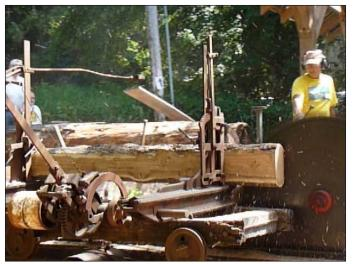
Guild Member Cory Colburn creates boards with his 52" circular saw blade powered by a cement truck. He finds 3rd gear works best. Picture taken at the Guild picnic in August.
