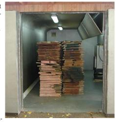
bility of the conditions on the inside of the chamber. The Nyle L200 system consists of several large fans, a central dehumidifier/heater/blower unit, and an externally located control unit. I found mine on eBay from an outfit that went
