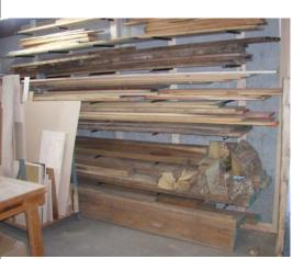
I angled the holes upward so when the pipes were inserted, a tiny bit loose, they were level when loaded. Be very careful in your own application. It is possible for the pipes to come out unless you
