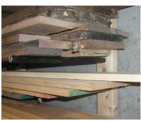
rack will hold 10-foot lumber easily The five 8-foot vertical supports have pipes spaced 12 inches apart, so that's 30 pipes to cut. If you have access to a metal cutting bandsaw you're in fat city.
