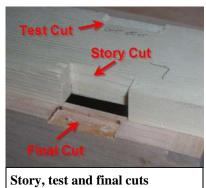
and/or lid , barely leaving a mark. Then set the router to final depth and re-cut it if the test is good.
