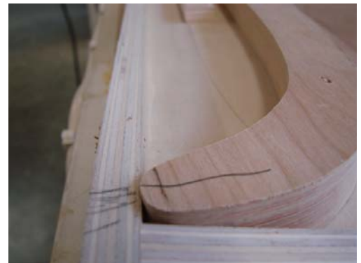
Figure 12 – marking for inside curve wedge
