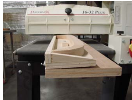
Figure 11 – sanding the wedge shape
